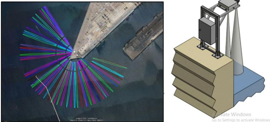
Figure 11. (a). Preferred jetty for installation of the Taranto tide gauge, showing a Fresnel zone (footprint for GNSS-IR) for one possible location (b) Proposed design of tide gauge framework and sea level instruments showing downward-projecting radar sensors
