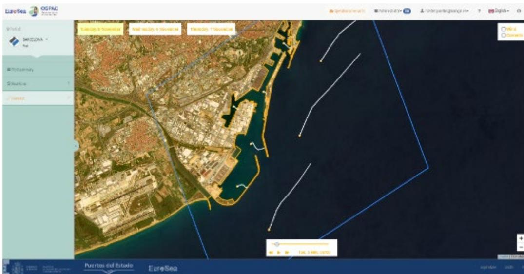
Figure 24. Forecasted floating debris trajectories at the Barcelona harbour, derived from the currents from the downstream CMEMS model. The orange dots represent the source origin of the floating debris (defined by the Administrator). The solid white lines are the lagrangian trajectories at different points inside/outside the Barcelona harbour.
