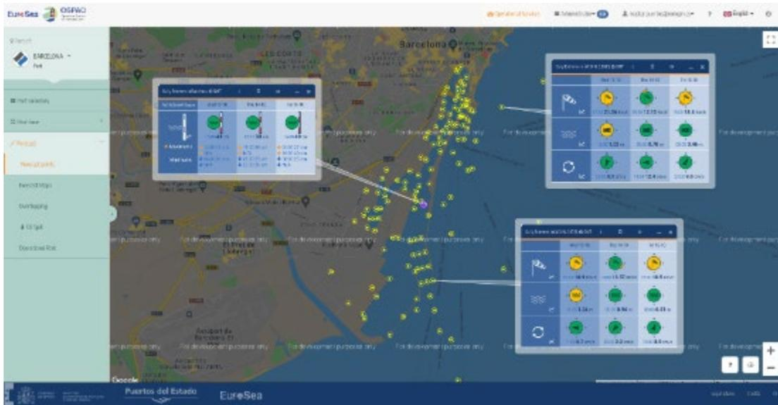
Figure 23. Screenshot of the OSPAC application (Desktop version). Forecast points at several points of the Barcelona harbour for the following met-ocean parameters: sea level (left); wind, waves and currents at the harbour entrance (centre) and wind, waves and currents at the outer part of the harbour (right).
