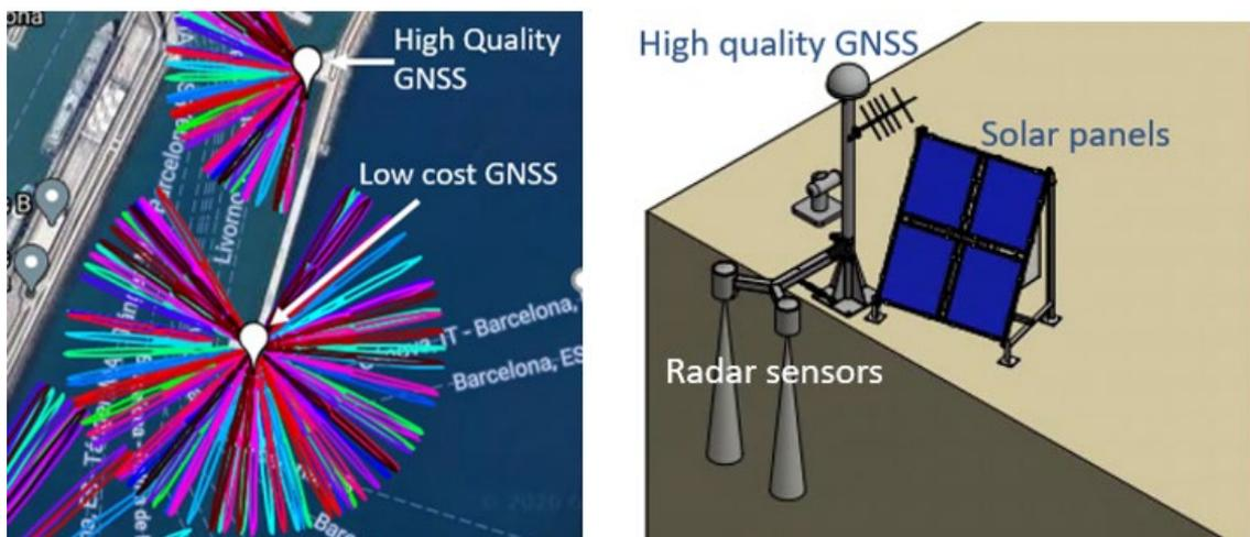
Figure 10. (a). Location for installation of the Barcelona tide gauge, with coloured radial lines showing a Fresnel zone (footprint for GNSS-IR) for the chosen locations of GNSS receivers (b) Proposed design of tide gauge framework and sea level instruments showing downward-projecting radar sensors and GNSS receiver.
