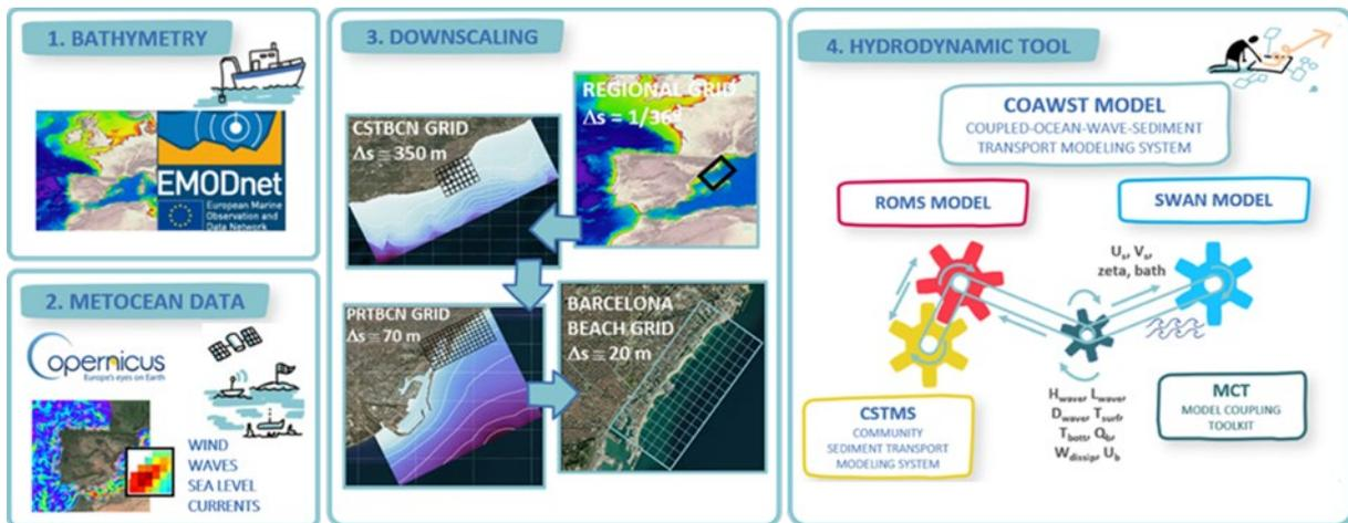
Figure 16. Hydrodynamic tool and setup overview scheme
