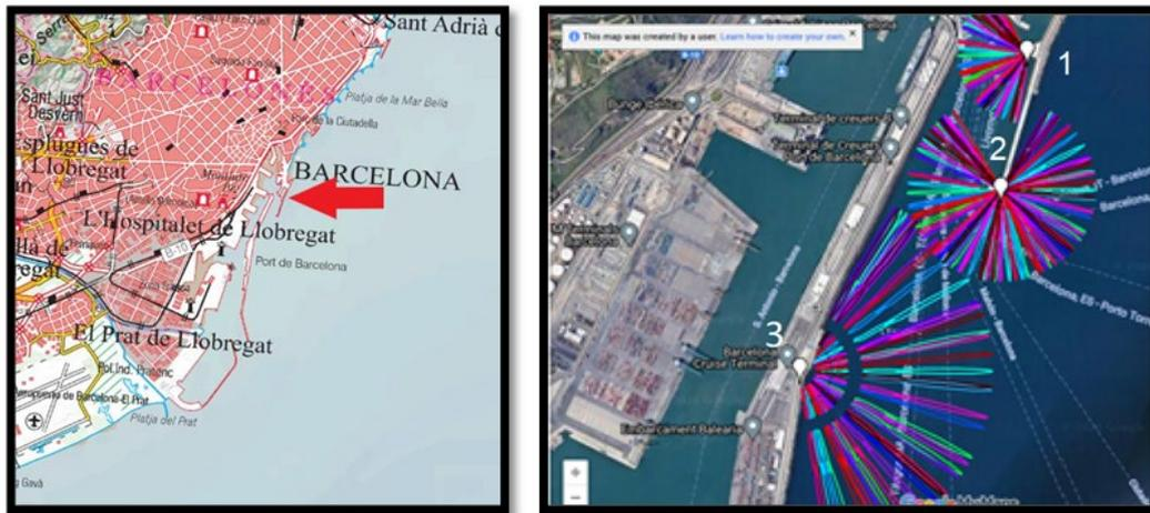
Figure 1. Area of interest for Barcelona tide gauge shown by red arrow (left) and specific sites shown by white markers (right). Radial lines denote the area of the sea surface that can be 'seen' by GNSS-IR technology at each location. These are also known as Fresnel zones.
