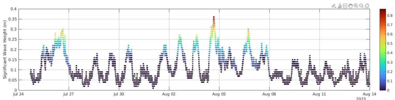
Figure 19. Significant wave height from the MIROS radar sensor at Taranto
