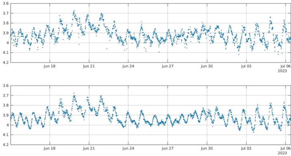
Figure 14. Sea level from GNSS-IR (top) and conventional radar sensor (bottom) at Barcelona Site 1
