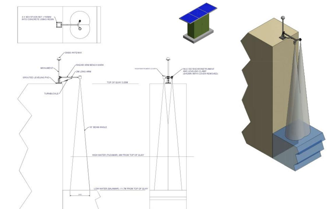
Figure 7. 2-D (left) and 3-D (right) representation of the agreed tide gauge design for Buenaventura. The solar panels are shown mounted on the upper surface of the electronics cabinet (in green)
