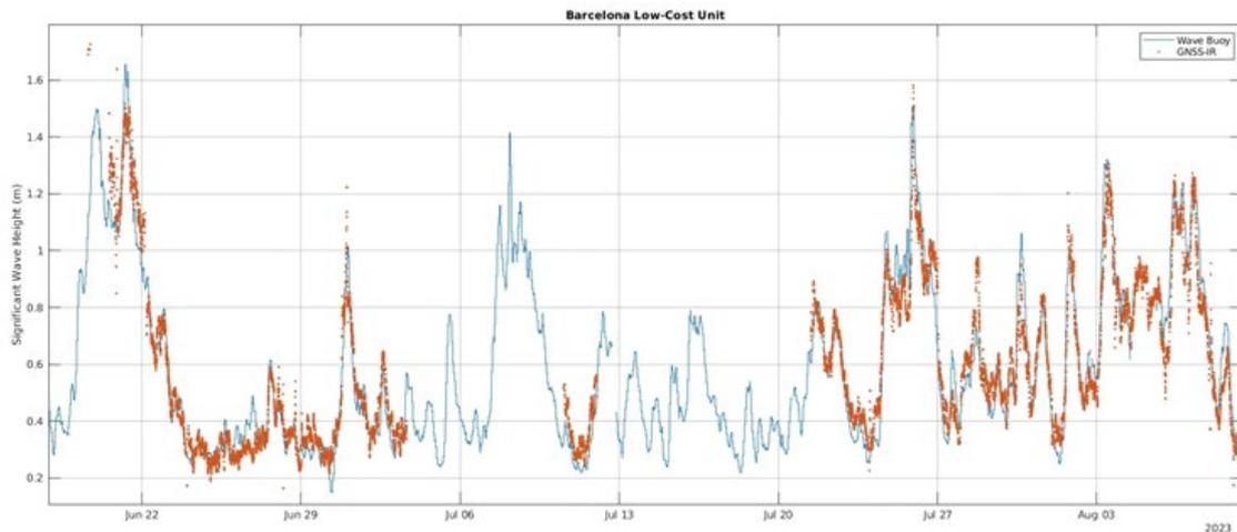
Figure 15. Comparison of SWH from GNSS-IR at the Barcelona lighthouse and an offshore wave buoy maintained by PdE
