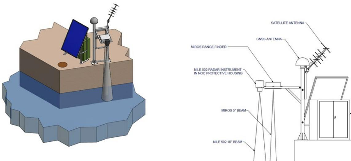
Figure 6. 3-D (left) and 2-D (right) representation of the agreed tide gauge design for Taranto
