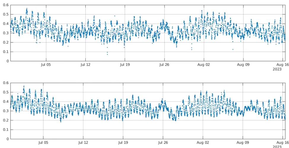
Figure 20. Sea level from GNSS-IR (top) and conventional radar sensor (bottom) at Taranto
