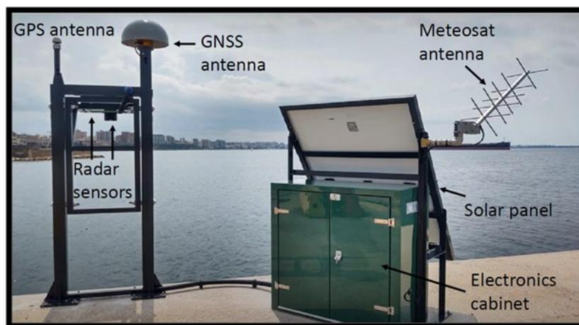
Figure 9. Completed tide gauge installation at Taranto
