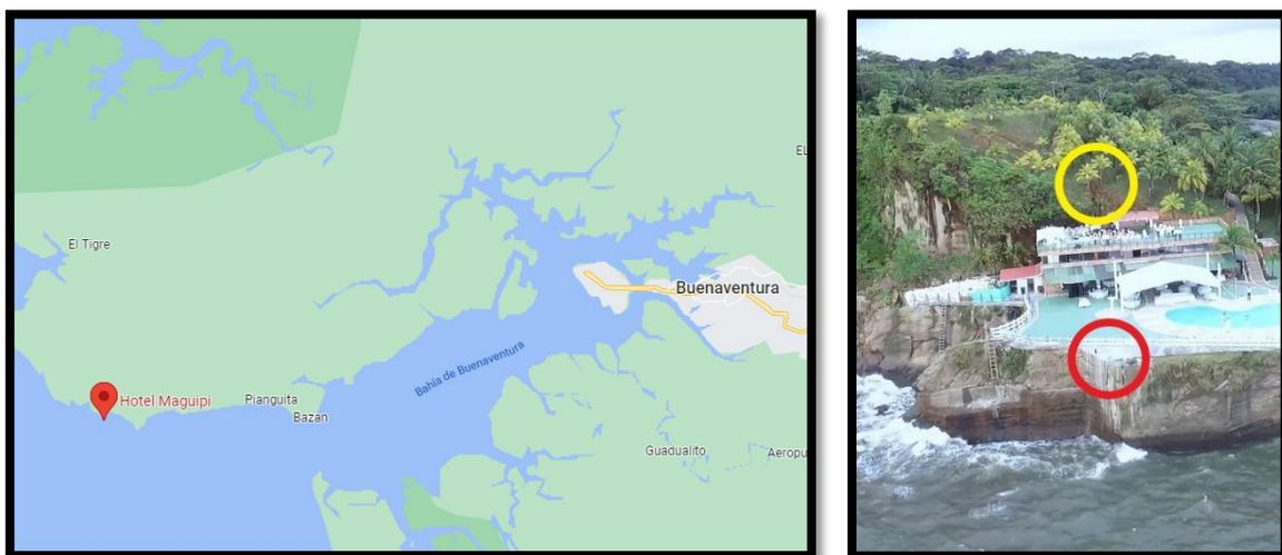
Figure 4. Agreed site for Buenaventura tide gauge installation at Hotel Maguipi. The right panel shows the planned location of sensors (red circle) and the supplementary electronics (yellow circle)
