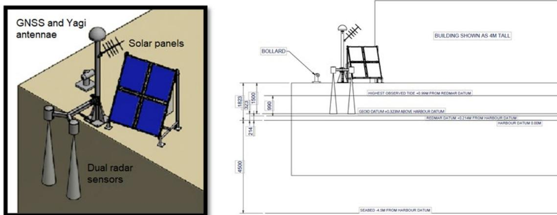
Figure 5. 3-D (left) and 2-D (right) representation of the agreed tide gauge design for Barcelona
