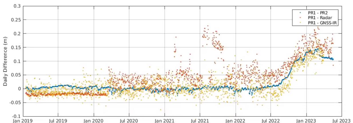
Figure 3. An example of data channel intercomparison (by differencing) for the Gibraltar tide gauge. PR1 denotes pressure sensor 1, PR2 denotes pressure sensor 2.
