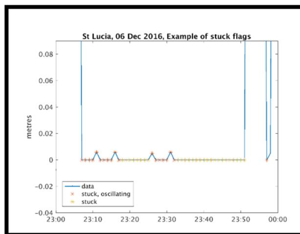
Figure 2. An example of stuck oscillatory sea level data
