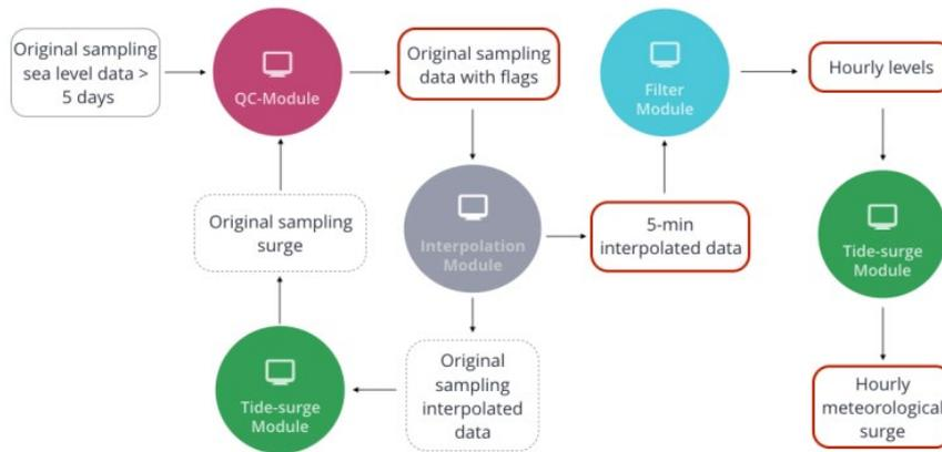
Figure 1: SELENE modules (QC, Interpolation, Tide-Surge and Filter) and data flow of the software. The final output products are framed in red and consists of the original sampling data with added data flags, 5-min interpolated data, hourly sea levels and residuals (aka meteorological surge component) (Pérez-Gómez et al, 2013).
