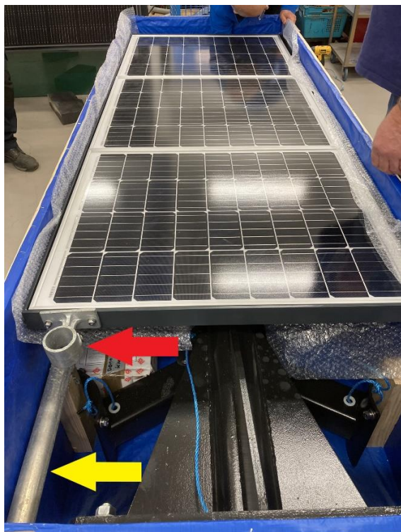
Figure 30 Yagi antenna mast (yellow arrow) and mast clamp (red arrow).
