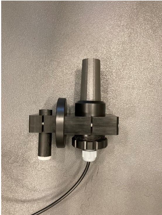
Figure 10 Radar antenna and mounting bracket.
