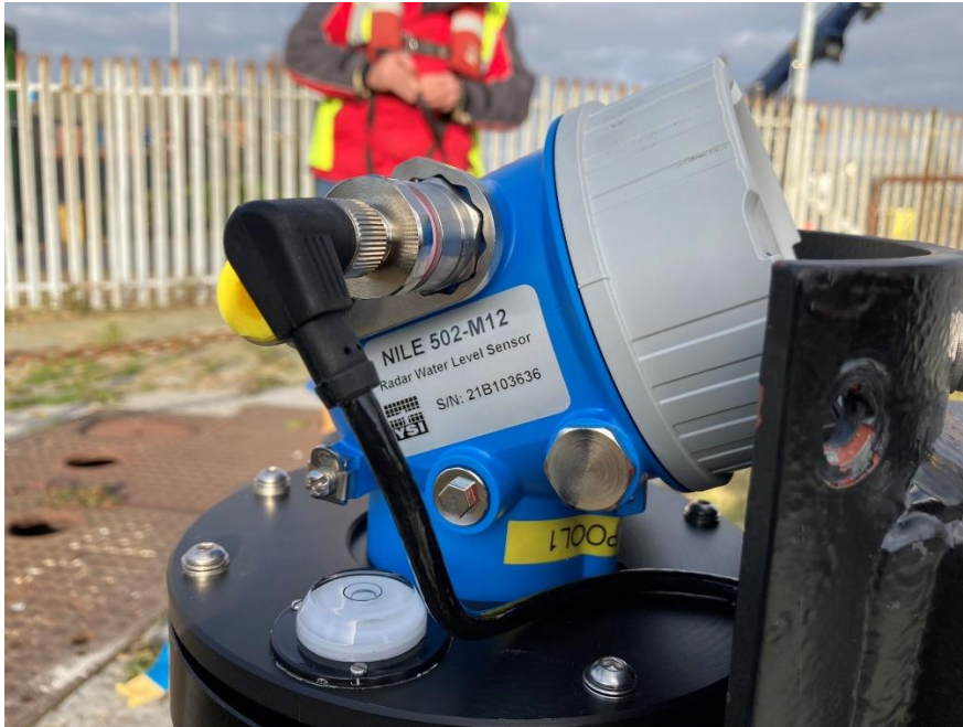
Figure 18 Radar sensor showing bubble level and adjustment screws.
