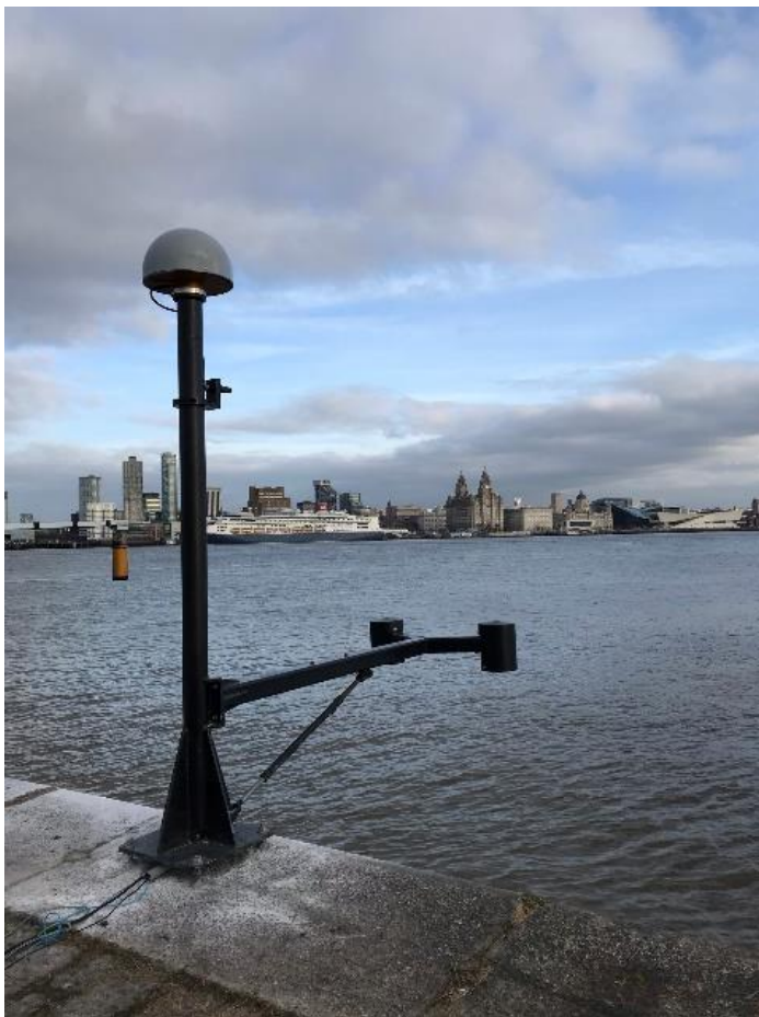
Figure 7 Radar arm in the outwards position.
