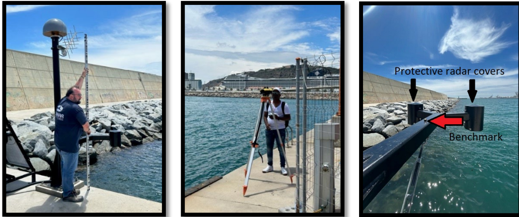
Figure 4. Jose Maria (SIDMAR) holds the levelling staff on the TGBM (left), whilst Yosamy estimates the TGBM height using the optical level (centre). The additional benchmark on the radar arm is shown (right)
