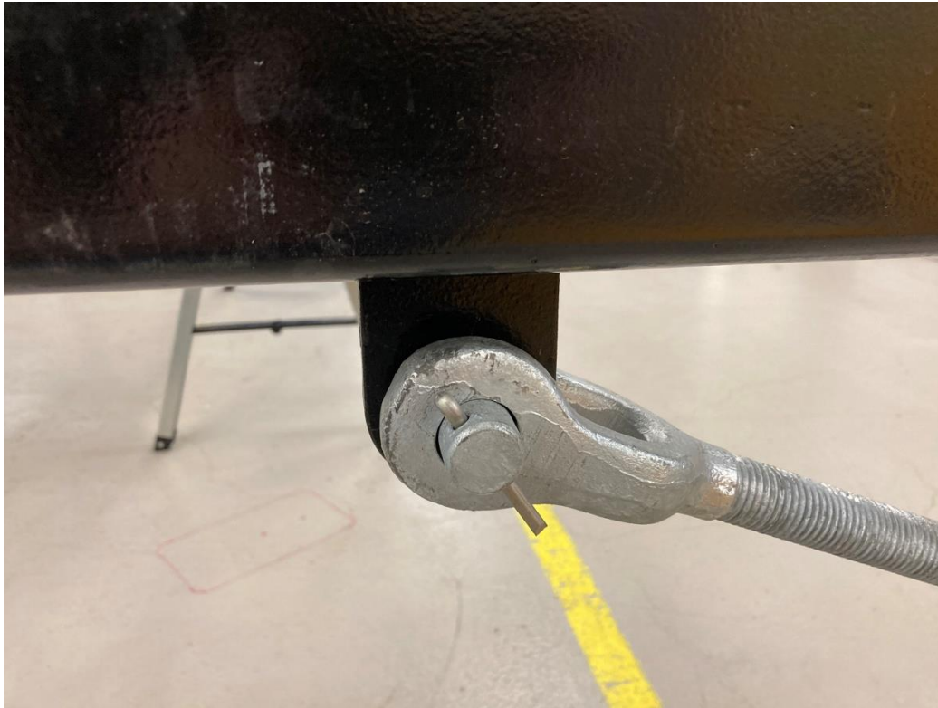
Figure 52 Turnbuckle attached to the radar arm.
