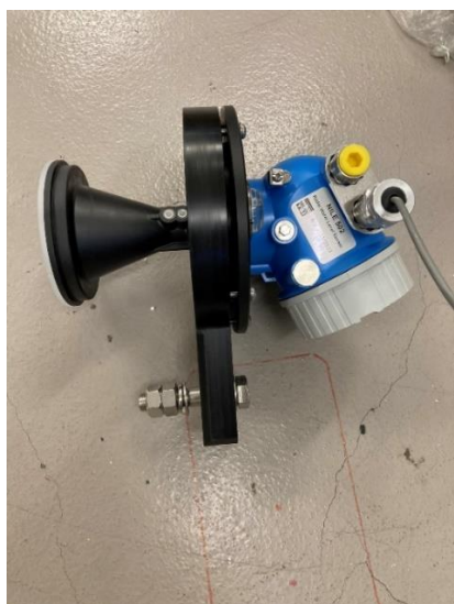
Figure 21 Radar sensor attached to mounting clamp.
