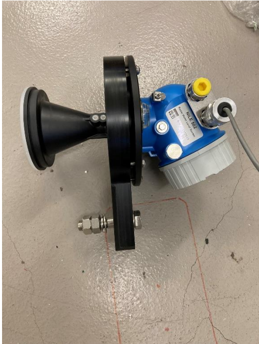
Figure 16 Radar sensor attached to mounting clamp.
