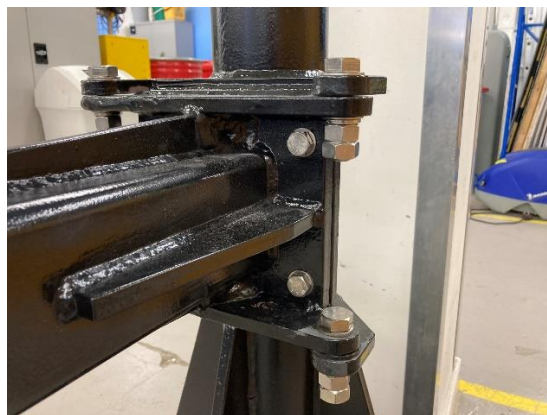
Figure 20 Radar arm mounting bolts.
