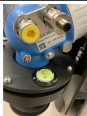
Figure 11. Levelling bubble on Nile radar
