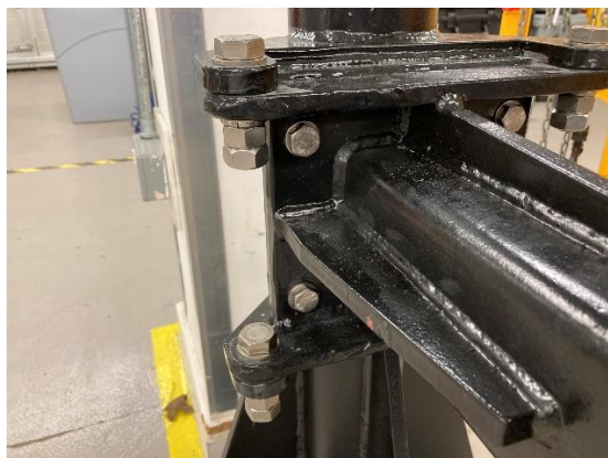
Figure 19 Radar arm mounting bolts.
