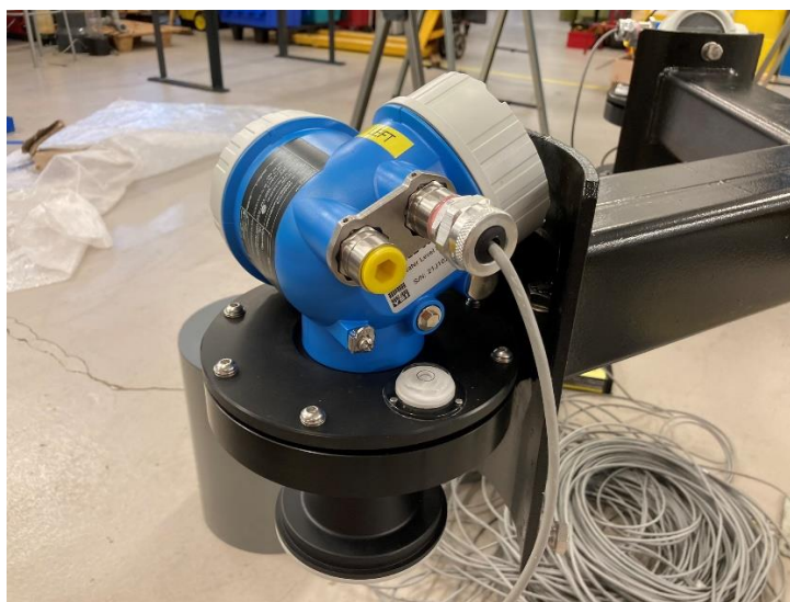
Figure 22 Radar sensor fitted to radar arm.
