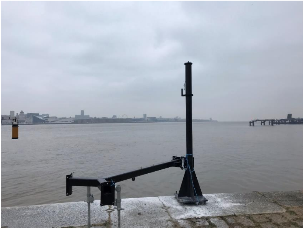
Figure 6 Radar arm swung inwards at Alfred Dock. Barcelona radar arm will swing inshore from the right side.
