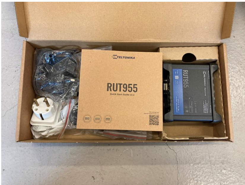
Figure 48 4G Modem RUT955 for lightning detector.
