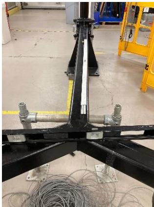
Figure 25 Levelling the radar arm.
