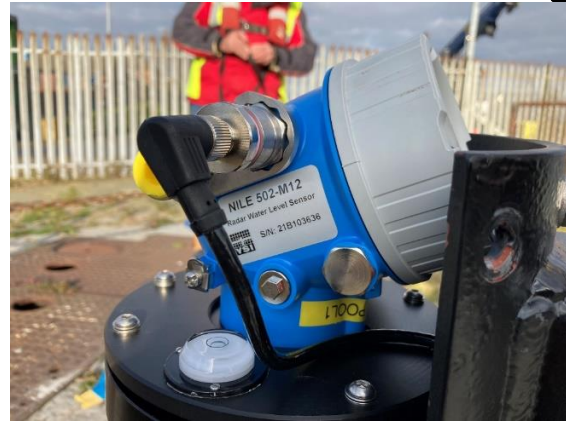
Figure 24 Radar sensor showing bubble level and adjustment screws.
