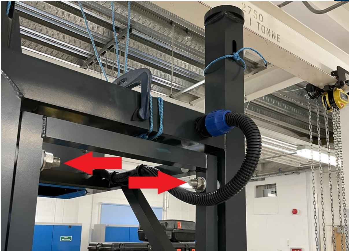
Figure 7 A frame swing arm installed.
