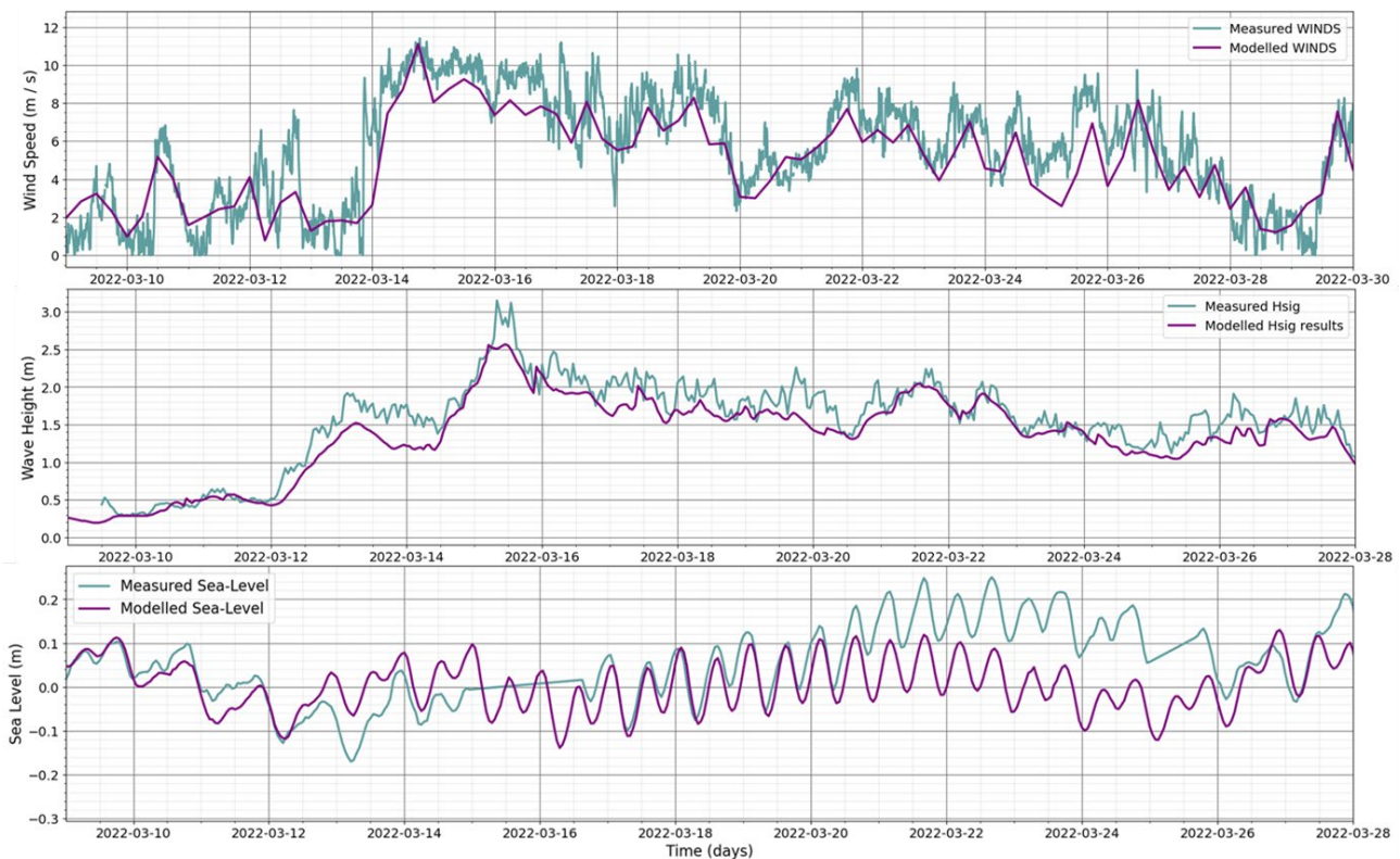
Figure 15. Comparison between measured data (in green) and modelled outputs (in purple) at the black dot location (see Figure 11). The upper panel shows time serie of wind speed (m/s), the central panel shows the time serie of significant wave height (m), and the lower panel shows the time serie of Mean Sea level (m).
