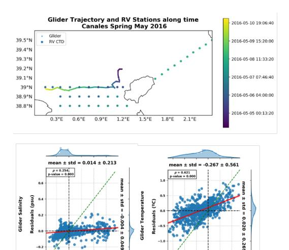
Figure 7. Top: A sample trajectory of a glider in the western Mediterranean Sea overlaid by the CTD sampling locations used for validation. Bottom: Comparison of the innovation and the residual for the salinity (left) and temperature (right) from the WMOP
