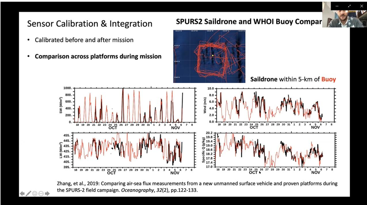
Figure 28. SPURS-2 best practices related to sensor calibration and integration between ASV Saldrone and moored buoy conducted by NOAA.
