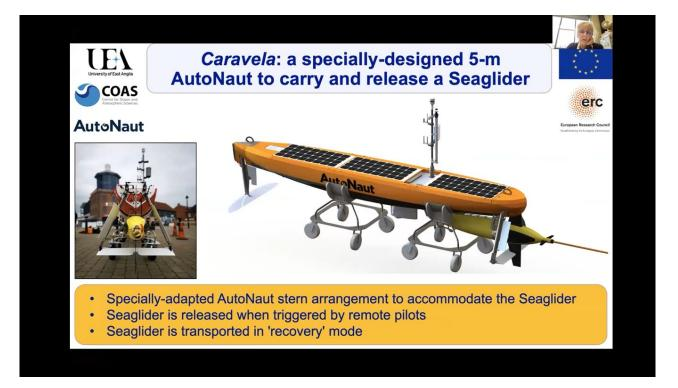
Figure 13. Caravela – A synergistic project between ASV and underwater glider technologies conducted by UEA.
