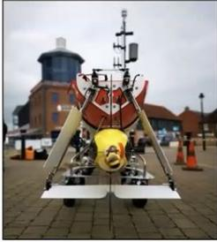
**Caravela: a specially-designed 5-m AutoNaut to carry and release a Seaglider**
