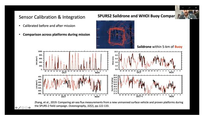
Figure 28. SPURS-2 best practices related to sensor calibration and integration between ASV Saildrone and moored buoy conducted by NOAA.
