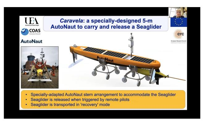
Figure 13. Caravela – A synergistic project between ASV and underwater glider technologies conducted by UEA.
